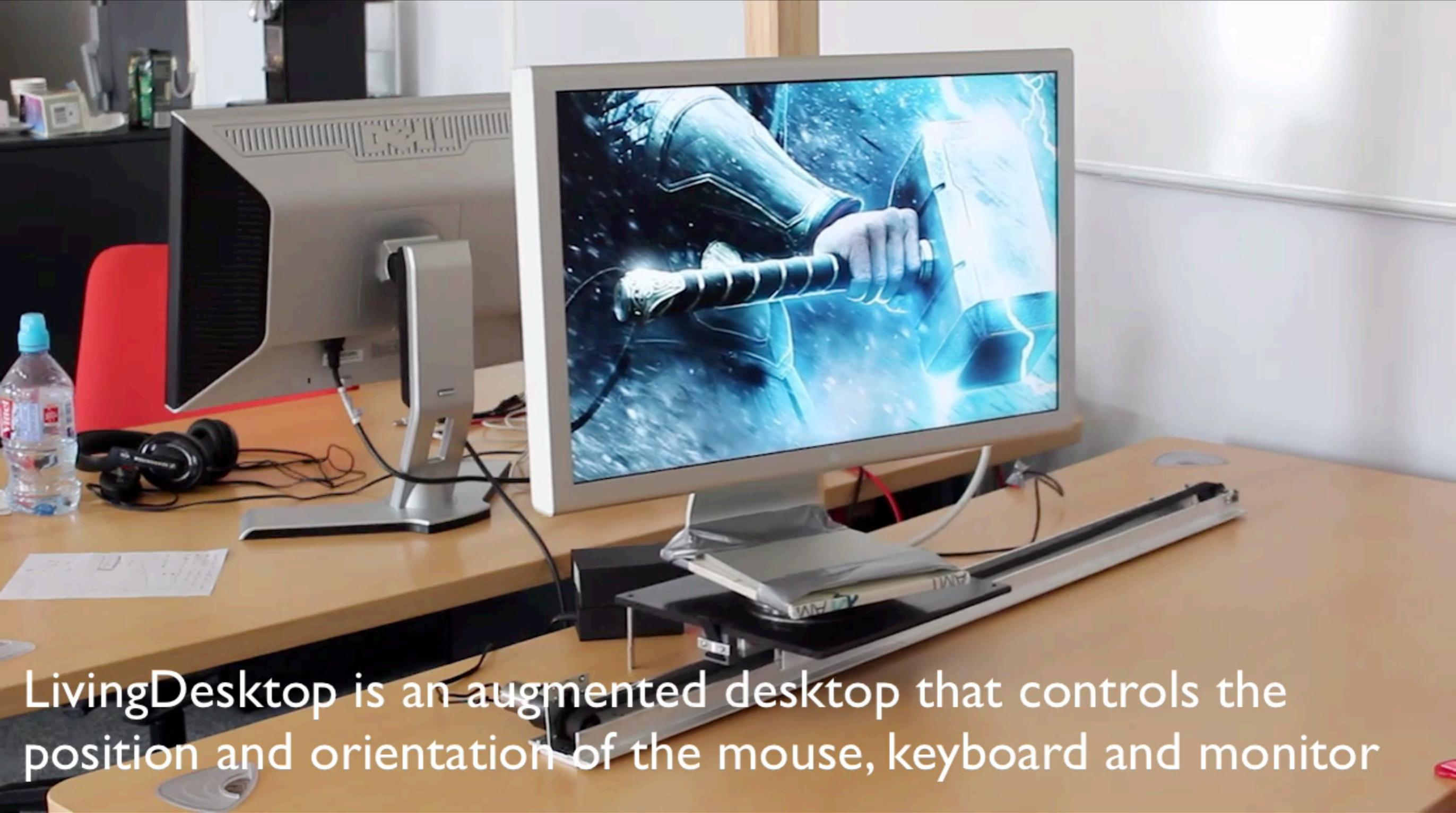
LivingDesktop is an augmented desktop that controls the position and orientation of the mouse, keyboard and monitor
