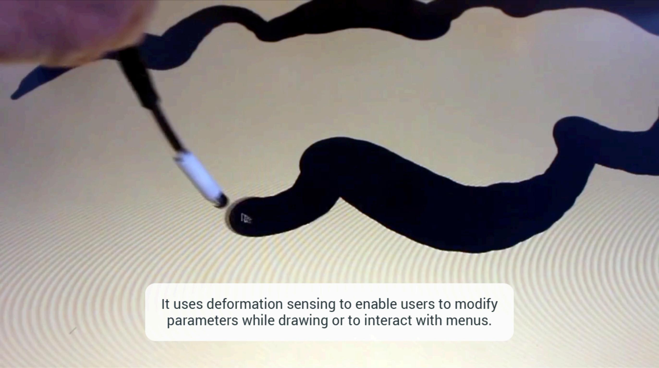
It uses deformation sensing to enable users to modify parameters while drawing or to interact with menus.
